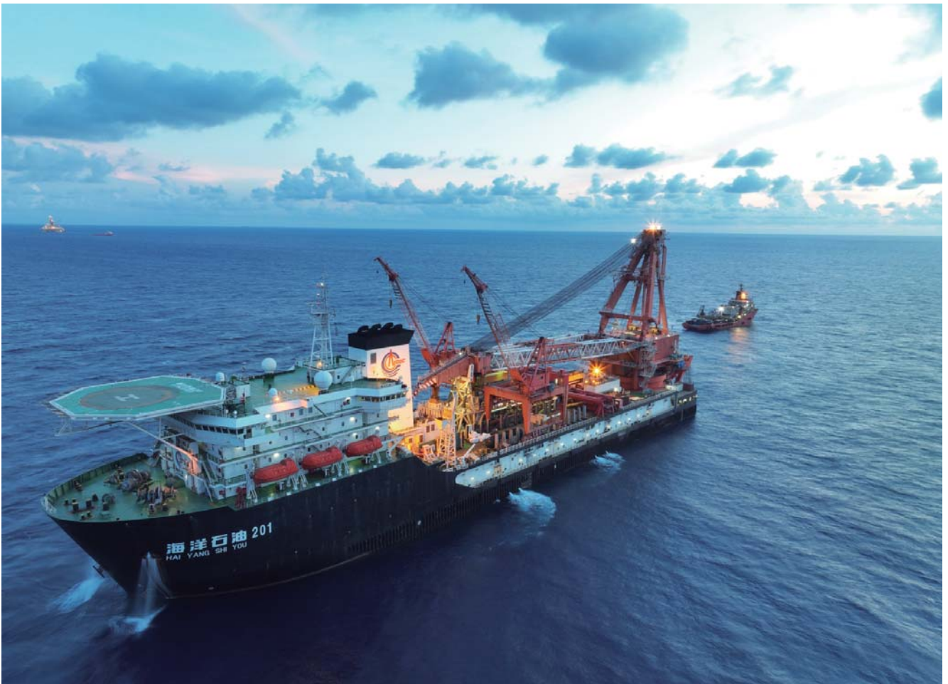
The Phase-II Lingshui 25-1 Project of "Shenhai-1" - Marine pipelaying
