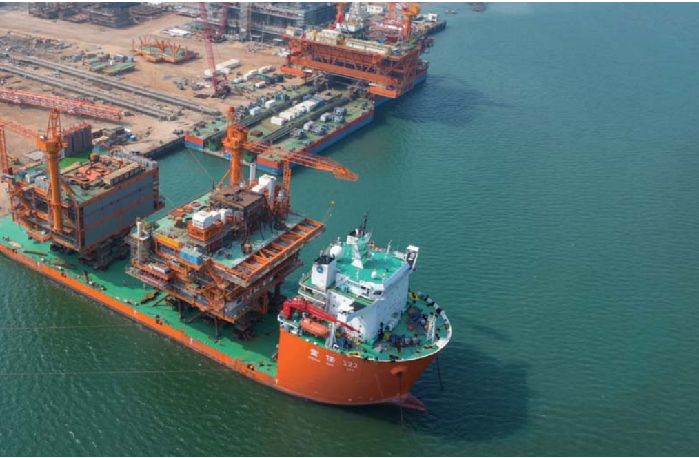
Module shipment and sailing in Lufeng Oilfield Phase-II Development Project
