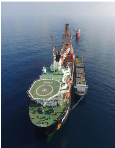
深水/超水深海管铺设 Deepwater Pipelay
