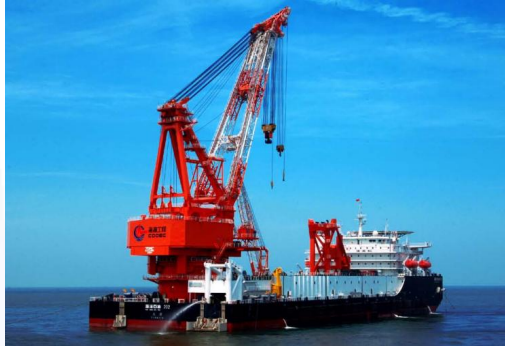
HYSY202 Derrick & Lay (1,200tons)
