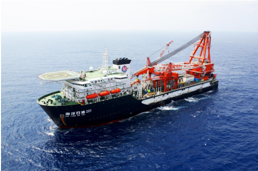
HYSY201 Derrick & Lay (DP3, 4,000tons)
