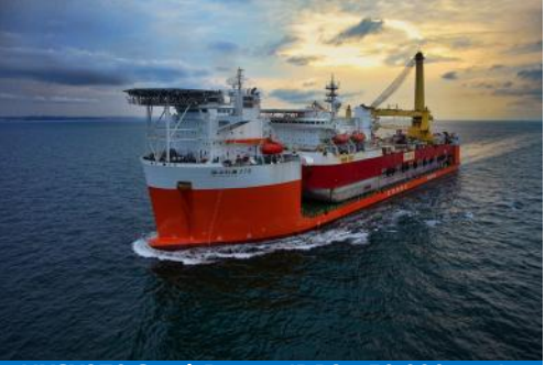
HYSY278 Semi-Barge (DP2, 50,000tons)
