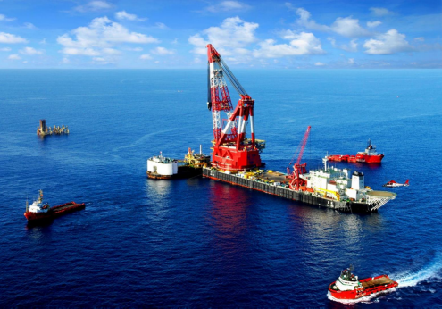
Lanjing 7500 Derrick (7,500tons)
